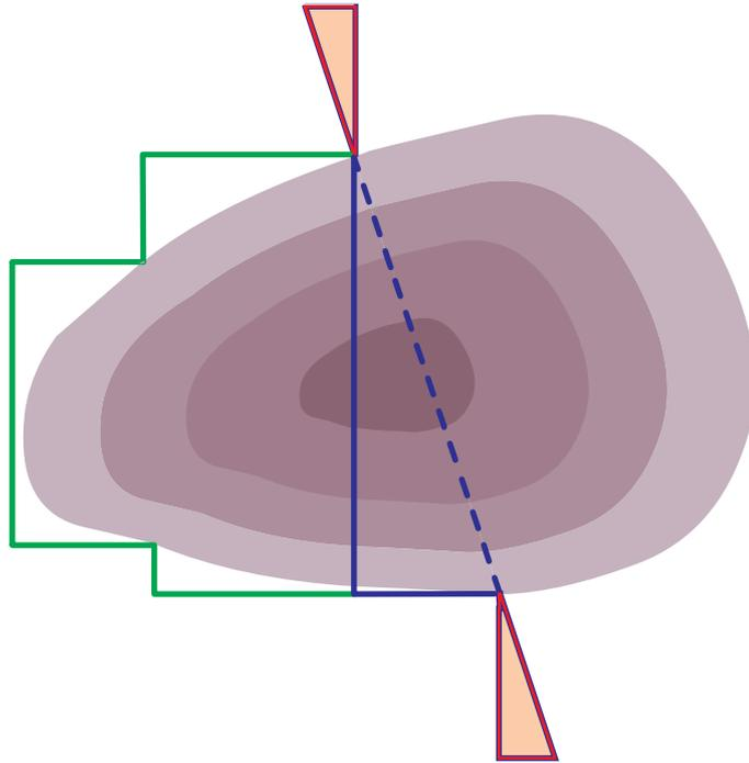
*By measuring the net distance traveled in each of two perpendicular directions, the lengths of two legs of a right triangle are determined, and the hypotenuse of the triangle is the proposed line of the tunnel. By laying out smaller similar right triangles at each entrance, markers can be used by each crew to determine the direction for tunneling. (T. Apostol)*
